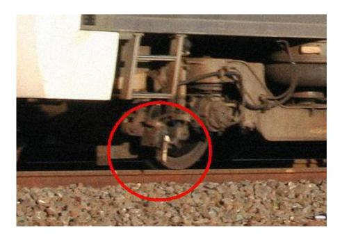
the trip arm in the raised position, the trip arm makes mechanical contact with the trip cock on the train, causing the train's brakes to be automatically applied, thereby bringing the train to a halt.
