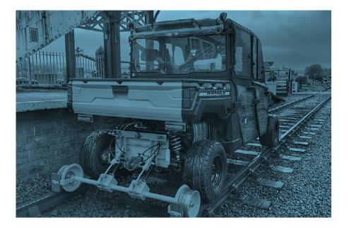
Legislative requirements mandate that the machine is CE marked. RIS-1530-PLT requires that the harmonised standard for RRVs, BS EN 15746- 2:2010+A1:2011, is used. Although CE marking is fulfilled by the manufacturer self-certifying the machine, this is also reviewed in part during the PA process.
