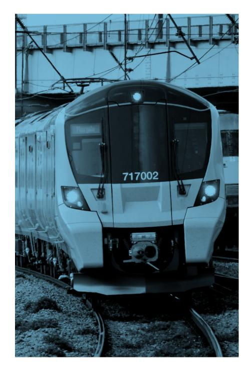
To align with Network Rail's roll out of ERTMS on the ECML, the scope authorisation for the Class 717 units authorisation needs to be increased to include ETCS Levels 0, 1 and 2. This requires authorisation of the Class 717 CCS subsystem to enable the additional.
