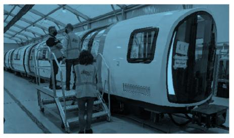
A key activity for the safety assessment of this project stage was the safety audit undertaken by ACS at the new test facility at Edmiston Drive, Glasgow. The stabling depot and test track allows the new 3-car metro trains to be tested with the intearated signalling system supplied by Stadler's project partner Hitachi STS. The ACS ISA team undertook a walkthrough inspection of a test unit, interviewed test and commissioning staff and witnessed a typical test activity on the test track.
